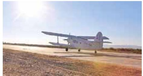
Feihong-98 (FH-98) is now the world's largest unmanned transport aircraft, with a maximum payload of up to 1.5 tonnes, it said. It was adapted from the prototype of the Shifei Y5B, a China-developed transport plane. As China's first fully domestically-built transport aircraft, the Shifei Y5B has a history of over 60 years since its first flight in 1957 and has been widely used.
